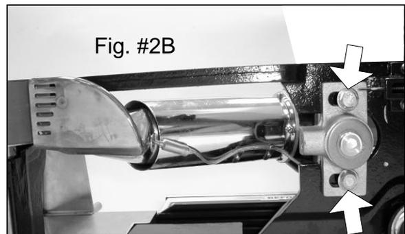
**Checking the Compression Wheel:** Check the distance between the vertical centerline of the compression roller and the tip of the nozzle. The distance should normally be 2 1/4"-2 1/2" (55-60mm) from the centerline of the roller. Fig. #2B, Fig. #2C.
