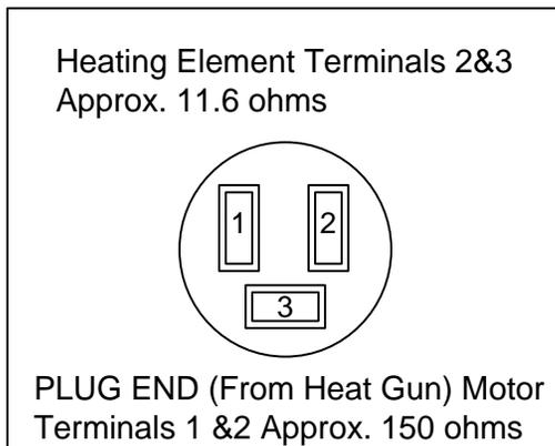
Fig. #16 Heat Gun Ass'y connector
