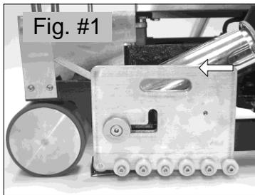
During use, it may be necessary to lubricate the wheels on the air dam by spraying the wheels with a silicone lubricant or WD-40. Rotate the wheels to assure that they move freely, then wipe any excess lubricant off the surfaces. Fig. #1 showing the air dam installed. To lower the air dam wheels on to membrane push the air dam toward compression wheel.
